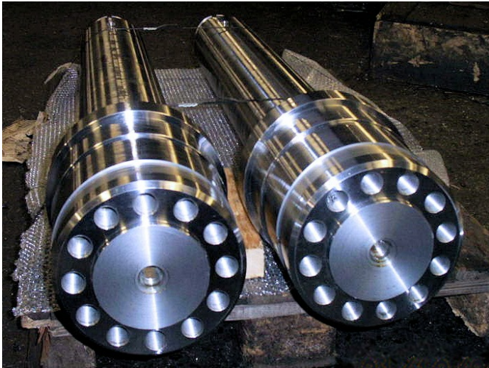
EN19(709M40) 270MM DIA. X 1450MM SHAFT
